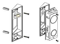
B. Install the angle adjustment bracket with 0.75" self-tapping screws.
